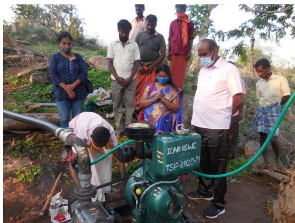
Diesel pump provided for lift irrigation
