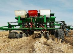
**ii.** <u>**Happy seeder:**</u> it is a PTO-driven machine with attached flails/blades for cutting stubble at the front and a hoe sowing system.
